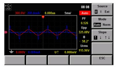
Figure 5.2: Trigger Setup Screen
