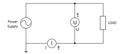
Figure 1.4: Low Current Wiring Setup
