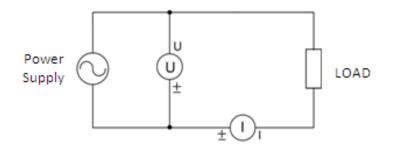
Figure 1.5: High Current Wiring Setup
