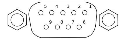
Figure 1.6: External Sensor Interface: DE-9 Connector
