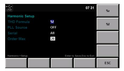
Figure 6.1: Harmonic Measurement Setup Menu
