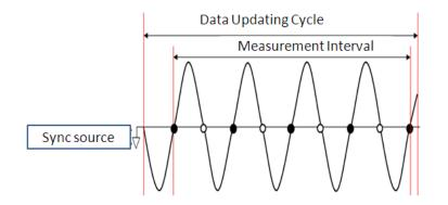
Figure 3.1: Measurement Timing
