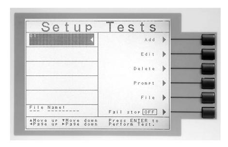
The Setup Tests screen is the central starting point for programming tests into the instrument. From this screen test parameters are entered and edited, and the order of the test steps is arranged. The 620L is capable of performing a 30-step sequential test from a single test file.
