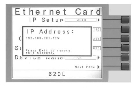
If the 620L fails to receive an IP Address after approximately 20 seconds, the following pop-up message will be displayed:
