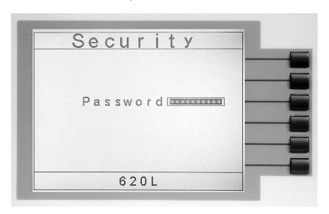
If a password has already been created the Security Password screen will appear and you must enter the correct password to access the Security Setting screen. From the password-protected Security Setting screen, three different parameters may be accessed: Change Password, Security and File Recall. The Security Setting screen
