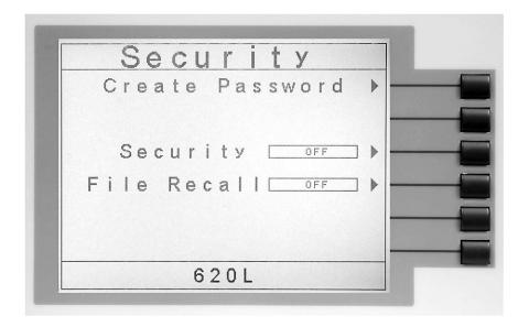
You may create a password from this screen so that all security functions will require a password. From the Security Settings screen, three different parameters may be accessed: Create Password, Security and File Recall.
