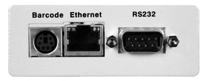
The port labeled "Barcode" is a PS/2-type connector that is used for the connection of a barcode scanner. The Ethernet port is for use with a standard CAT-5 Ethernet cable and may be connected to any compatible PC. The 9-pin D-type subminiature connecter labeled "RS232" is for connection of the 620L to an RS-232 communication bus.
