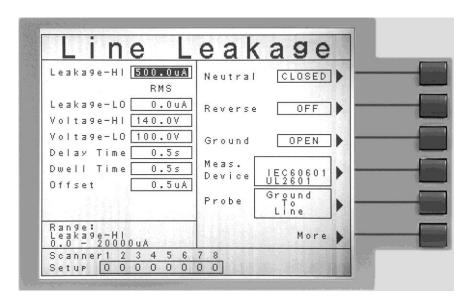
The user must then set the parameters for the line leakage test. When the Offset option is installed, the offset selection can be viewed from the Line Leakage parameters screen.
