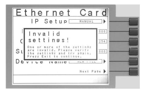
Press the EXIT key to save the new settings. If the IP Setup parameter is set to AUTO, you do not need to enter a Subnet Mask manually.
