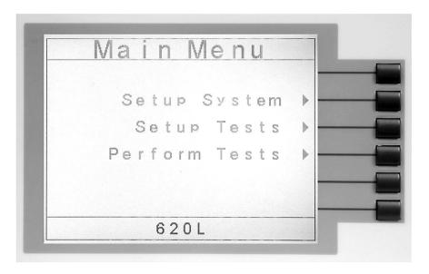
From the Main Menu screen three menus may be accessed: Setup System, Setup Tests, and Perform Tests.
