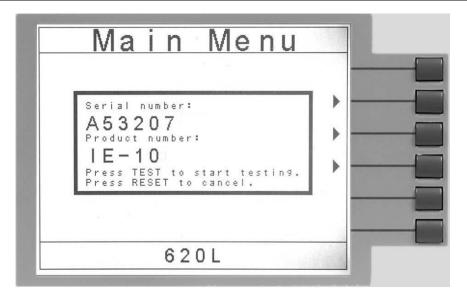
After the barcodes are scanned, press TEST to initiate the test sequence. Pressing RESET will abort the TEST sequence.
