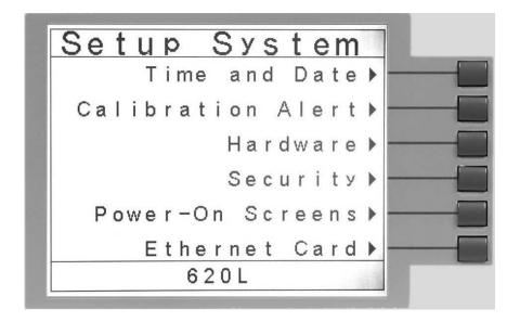
To access the Ethernet Card Menu, press the "Ethernet Card" soft key from the Setup System screen. The Ethernet Card Parameters screen will now be displayed as shown below:
