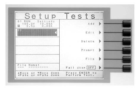
In order to delete a previously create prompt, use the up and down arrow keys to scroll the highlighted area to the step where you would like to delete the text prompt and press the "Prompt" soft key. The Prompt screen will now be displayed. Use the backspace key "←" to delete the text. Press the EXIT key to return to the Setup Tests screen.
