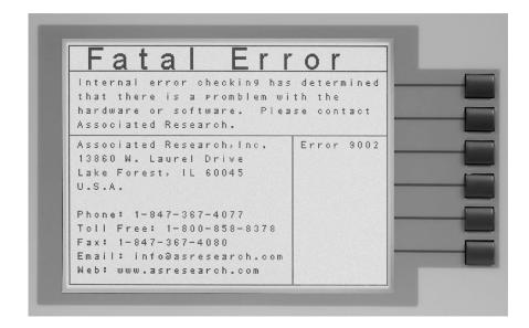
This type of failure permanently locks the instrument in the "Fatal Error" mode and requires that the instrument be serviced by Associated Research, Inc. The following Fatal Error identification numbers will represent the type of failure that has occurred:
