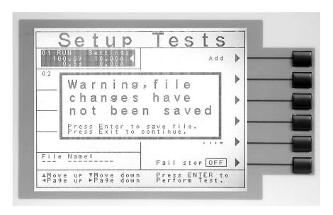
Pressing the ENTER key will store the file with the file name you gave it and go to the Perform Test screen. You may now perform a test (refer to section **5.3. Performing a Test**).
