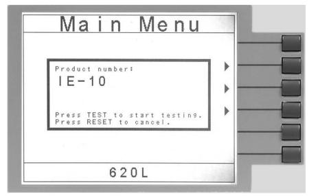
After the barcodes are scanned, pressing TEST will initiate the test sequence. Pressing RESET will abort the TEST sequence.
