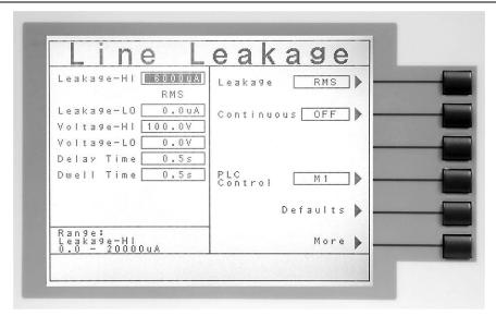
Setting the PLC Control selection to M1 through M7 will create different digital states at Bit 0, Bit 1, and Bit 2 of the PLC Remote Signal Output (refer to the PLC Signal Output drawing below). The different states are described in the truth table below. The "Not used" state is undefined and cannot be programmed for use.
