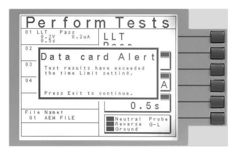
By pressing the EXIT softkey, the message will be cleared and it won't appear again until the unit is re-booted or the Time Limit setting is set to a different value.
