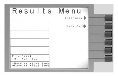
Pressing the softkey labeled Instrument will display the detailed results from the previously executed test file. Pressing the softkey labeled Data Card will display the Data Storage Card Results menu as shown below:
