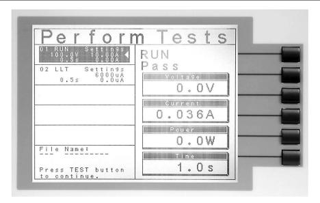
You may single step through an entire sequence in this way as long as you do not press RESET. Once RESET is pressed it will return you to the originally selected step.
