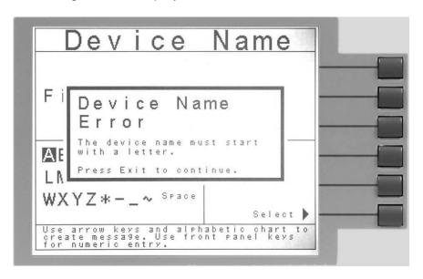
When the Device Name has been entered, press the EXIT key to save the new settings. The Device Name parameter is only active when the IP Setup is set to AUTO.
