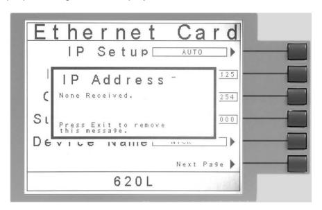
Press the EXIT key to remove the pop-up message and return to the 620L's Main Menu Screen.
