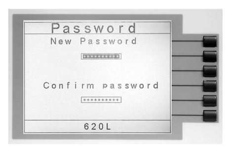
You may now type in the new password using the numeric keypad. Press the ENTER key to accept the new password or press the EXIT key to escape. After you type in your new password, you will be required to confirm your new password by typing it again into the "Confirm Password" field. Press the ENTER key to confirm the new password or press the EXIT key to escape.
