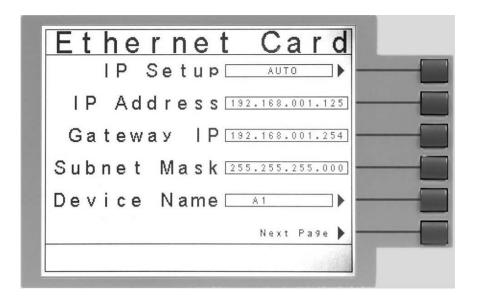
From the Ethernet Card Parameters screen, six different parameters may be accessed: IP Setup, IP Address, Gateway IP, Subnet Mask, Device ID, and Next Page.
