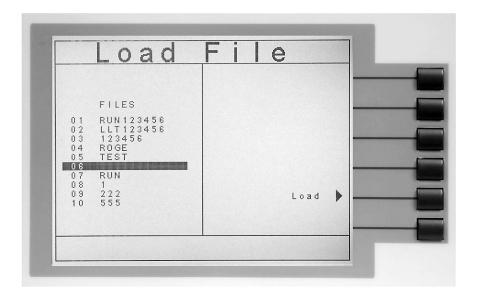
Using the up and down arrow keys, highlight the file you would like to load and press the "Load" soft key. The file you selected will now load and the screen will revert to the Perform Tests screen.
