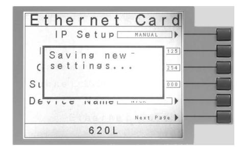
The Ethernet Card will attempt to re-establish a connection with the server anytime the user modifies a parameter and exits the Ethernet Card Parameters Menu or uses the command set at the end of this option description. Thus, if the IP Setup is set to AUTO, the Ethernet Card will request a new IP Address every time a parameter is edited and, as a result, the "Requesting IP Address. . ." message will appear.
