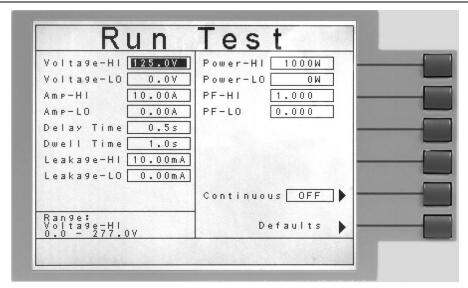
From the Run Test Parameter Setting screen the following parameters may be controlled: Voltage-HI, Voltage-LO, Amp-HI, Amp-LO, Delay Time, Dwell Time, Leakage-HI, Leakage-LO, Power-HI, Power-LO, PF-HI, PF-LO and Continuous. For detailed descriptions of these parameters refer to section **4.4.1. Description of Test Parameters**.
