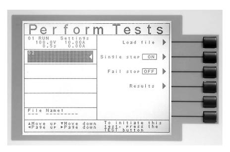
The Perform Tests screen is the main operational screen of instrument. From this screen individual steps are monitored while the test is being performed.
