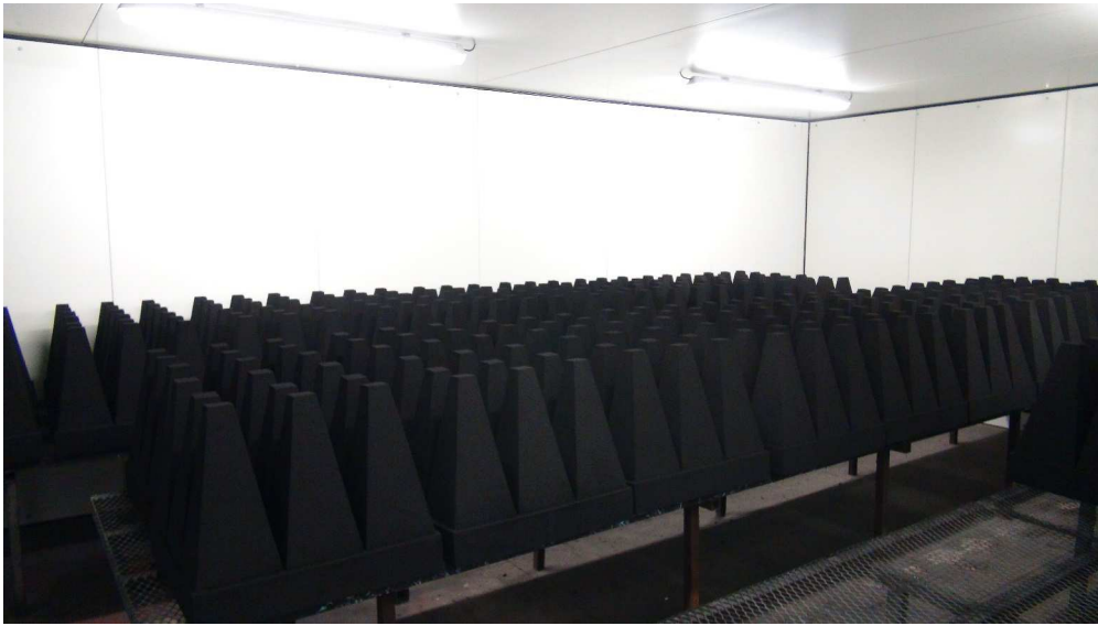
HPT Absorbers before painting
