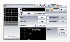
Measurement on PWM signals is included. Application: motors.
