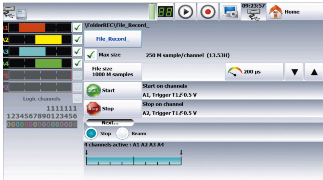
Trigger: several type of trigger, one channel, on a level, slope, several channels or combined conditions.
