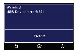
If the USB barcode device is removed while the instrument is powered on, the following message will appear:
