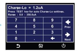
Enter <u>Charge-Lo</u> value to manually set Charge-Lo or Press TEST to perform auto Charge-Lo.
