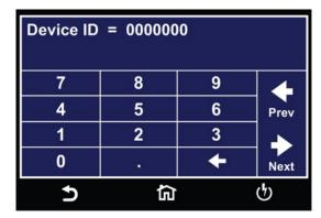
The Device ID number can be entered and saved using the touchscreen keypad.
