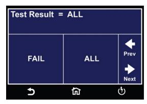
The two options available for Test Result are "All" and "Fail". This option allows you to select which test results will be printed. "All", selects printing all test results and "Fail only", selects printing only failed test results.
