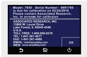
The above Calibration Alert screen will be displayed upon powering up the instrument, on and after the Calibration Alert Date. This screen will display the Calibration Due Date of the instrument.
