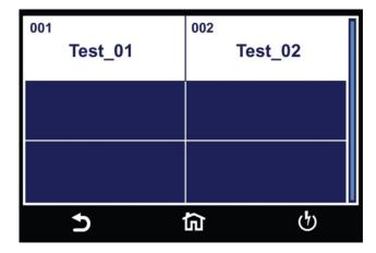
Load Test screen, if there are multiple test files saved in the instrument select the Load icon and all the test files will be displayed. You can select the test file and the first test step in the selected test file will be displayed.
