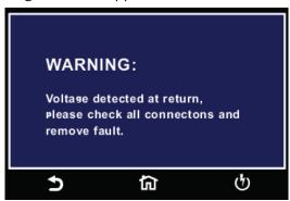
Check for any inappropriate connections to the Return line.
