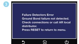
Ground Bond Fail Detectors ERROR screen.
