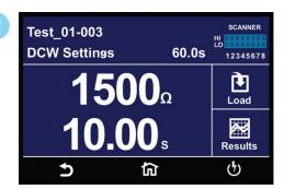
Perform Test Screen - Navigate to the Perform Tests screen in order to run a test sequence.
