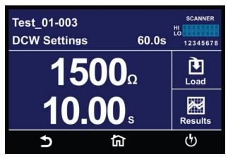
In the image above, the two large meters display the DCW test voltage and the Dwell Time.
