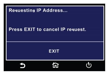
**NOTE:** The "Requesting IP Address..." pop-up message only appears at power up when the Ethernet Card has its IP Setup configured to AUTO.
