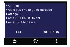
If there is a problem with the connection to the barcode reader or an incompatible device is plugged into the USB barcode port, the following message will appear:
