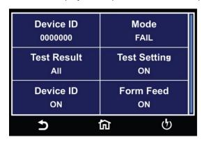
From the Print Format setting screen, six different parameters may be accessed; Device ID number, Mode, Test Result, Test Setting, Device ID, and Form Feed.
