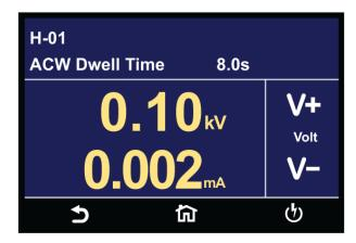
Pressing the "+" icon will increase the output voltage and pressing the "-" icon will decrease the output voltage. Manual voltage adjustment temporarily overrides the voltage setting and only remains in effect until the test is terminated by Pass, Fail, or Abort conditions. When Security feature is ON, manual voltage adjustment is disabled for users with limited access. You will not see the "+" and "-" soft key selections in this case.
