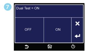
Select <u>Dual Test</u> ON or OFF for Dual Remote Palm Switches.
