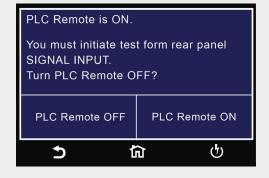
This screen comes up when pressing TEST button while PLC is ON warning customer to adjust PLC setting if need to use the TEST button.
