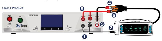
Did you know? If necessary, a 10 x 20 cm piece of foil can be attached to the enclosure to simulate a full hand contact to the DUT. This foil acts as the return point. The return and sense (-) terminal are attached to the foil. Always check to make sure you made a good connection between the DUT and the return clip.
