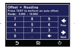
Enter <u>Offset</u> value to manually set Offset or Press TEST to perform auto offset.
