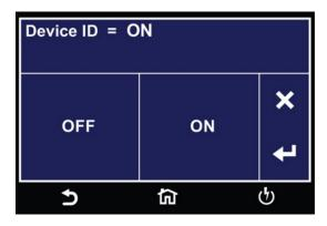
The Device ID number is a counter that increments once every time a test is performed. The number can be set to match the exact serial number or some portion of the actual serial number of the item under test, or just used as an identifier or tracking number. From the Print Format Setting screen select Device ID:
