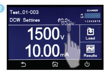
Touch and hold the display on any of the meters and drag it on to the location of a different meter and the two meters will be swapped.
