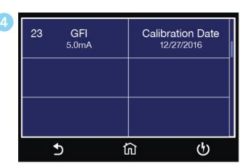
From the Calibration screens, use the touchscreen to select the parameter you wish to calibrate. A calibration prompt screen will now appear that describes the necessary load and connection information for the parameter being calibrated.
