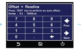
Enter Offset value to manually set Offset or Press TEST to perform auto offset.
