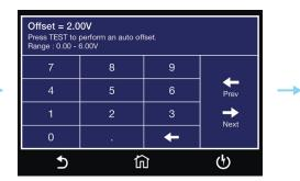
Enter <u>Offset</u> value to manually set Offset or Press TEST to perform auto offset.
