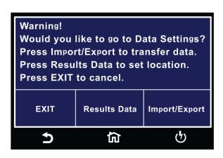
The Import/Export menu allows the user to import or export System and Test Files from a USB flash drive into the instrument memory. The Import/Export menu will only appear under the Hardware menu if a USB flash drive is inserted into the Data port on the front panel of the instrument.
