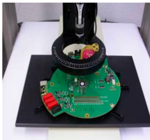
A circular solid state circuit board is mounted on the PCB holder and fixed with claw fasteners.
