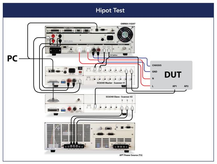
Figure 2 - Hipot Test Connections
