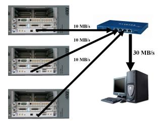
Figure 5: Data aggregation via gigabit switch
