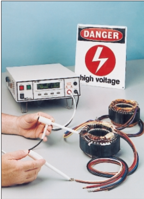
Operator tests stators with dual retractable test probes. Once released the high-voltage probes retract to prevent user contact with high voltage.
