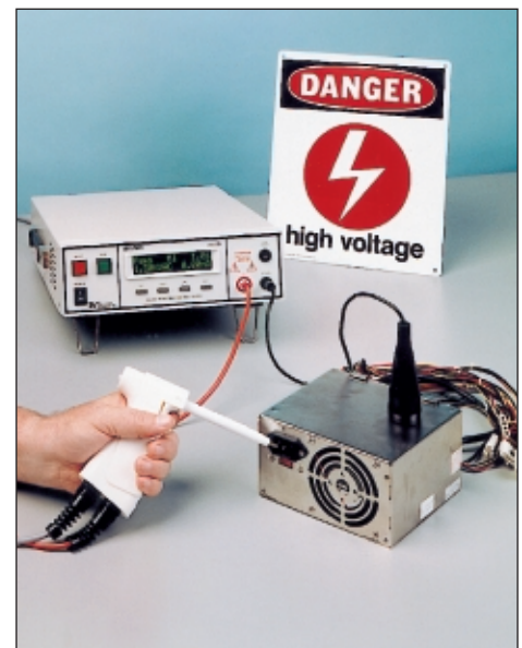
Operator uses a pistol style high voltage probe with the capability to automatically initiate the test by depressing the trigger. Activation of high voltage requires a two step action of retracting the probe shield and depressing trigger.
