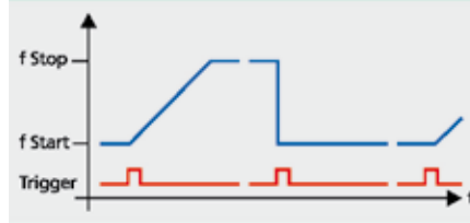
Triggered sweep with hold and triggered reset
