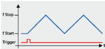
Continuous sweep with reverse after the start pulse
