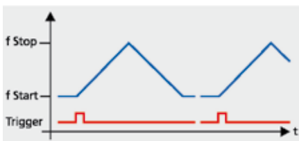
Triggered sweep with reverse
