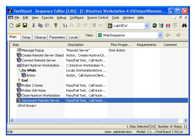
Huntron Remote Sample TestStand Program (RemoteControl.seq)
