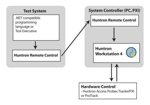
Remote Control through a separate controller
