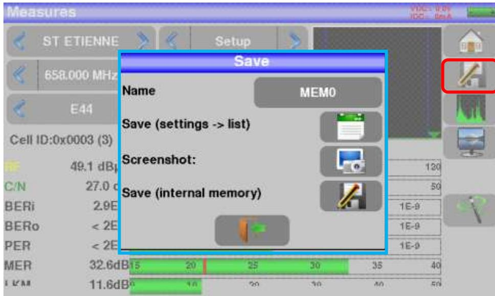
In this window, you can save the current measurement parameters from the active list, make a screenshot to a USB stick under BMP format or make a save into internal memory.
