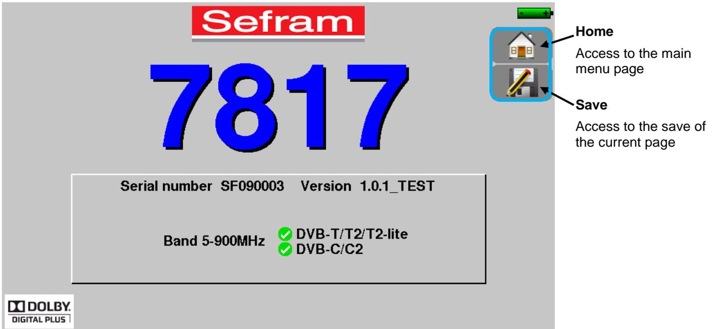
The Home page allows the navigation through all functions of the appliance. You will also find there the [Remote supply](#) and [Measures-TV-Spectrum](#) functions, the [AUTOSET](#), [Lists](#), [Library](#), [TERRESTRIAL check](#), [Configuration](#), [Constellation](#), [Echo Guard Interval](#) and [Measurement map](#).
