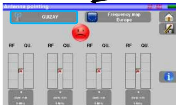
Enter 4 frequencies or channels of the transmitter you try to check.
