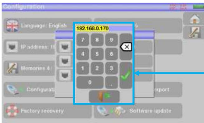
With the virtual digital keypad, type the IP address you want, then validate with ENTER
