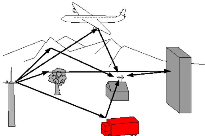
In digital TV DVB-T/H and DVB-T2, these echoes may help or degrade the image according to the time delay between the various signals that reach the antenna.
