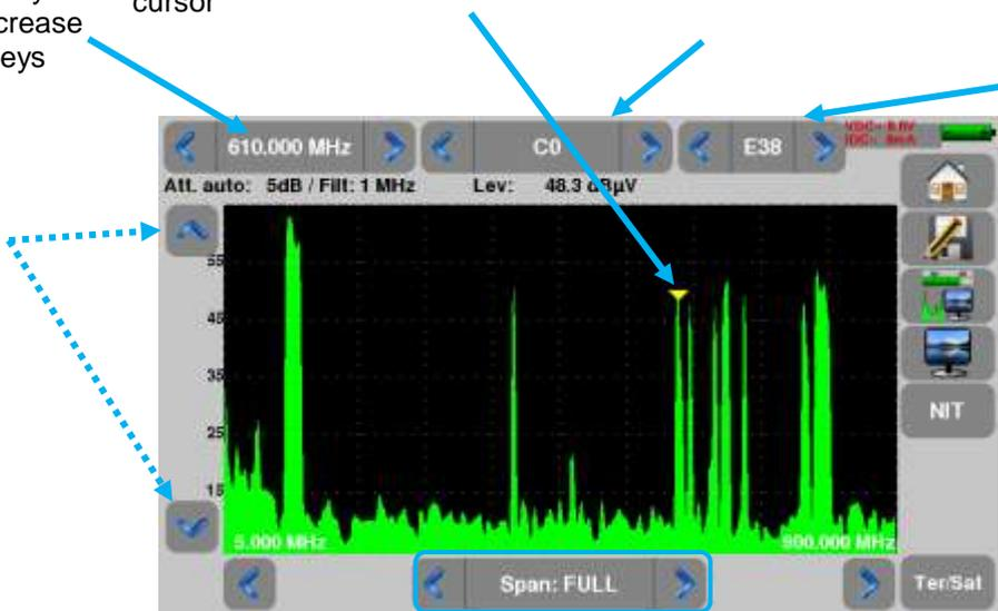
**Span :** frequency span around the center frequency
