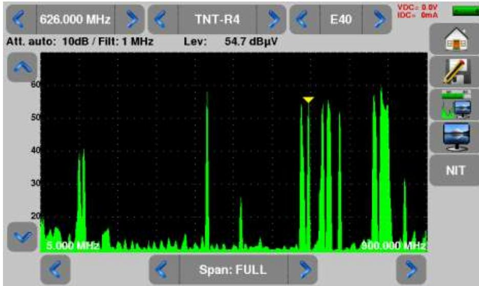
The input attenuator is automatically tuned according to the level of the signals measured.
