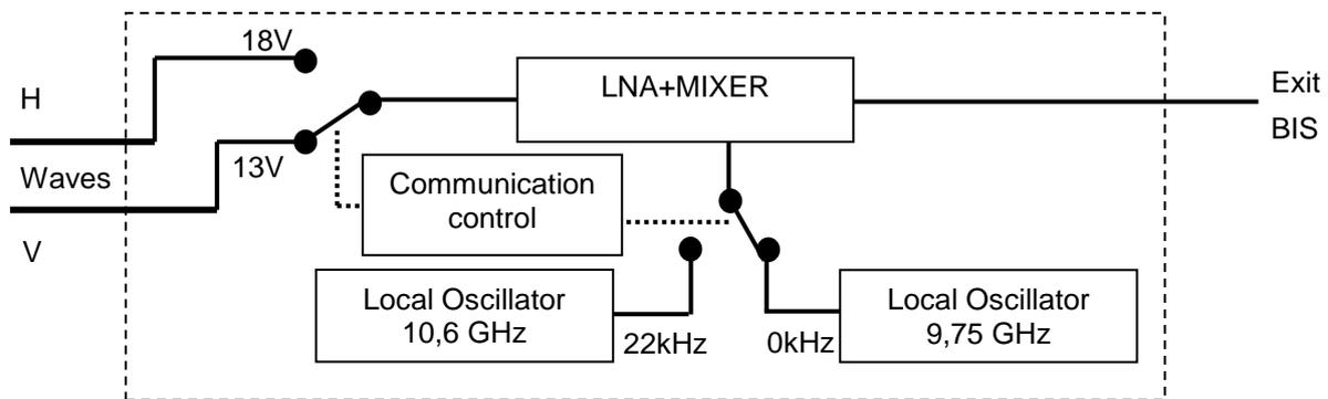
The reception is made on 2 low/high frequency band and 2 horizontal/vertical polarizations of the received wave.
