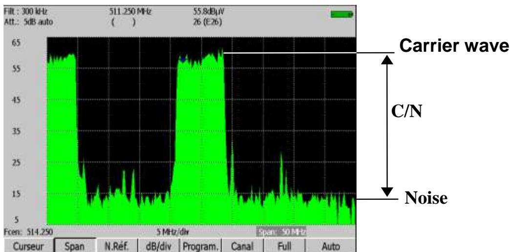
**COFDM**: Coded Orthogonal Frequency Division Multiplex.
