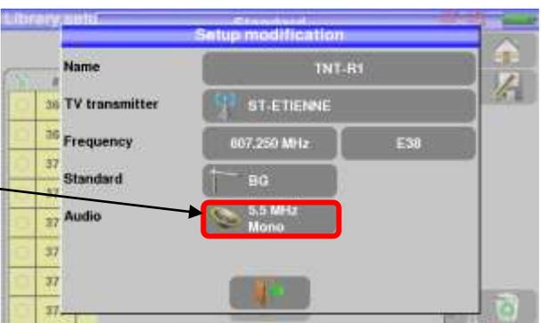
To enter the type of audio configuration you want for the setup (mono, stereo or NICAM)
