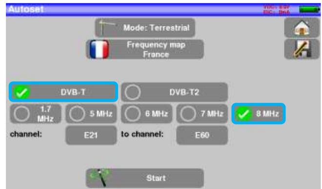
Press START. The appliance searches until the end of the scan and turns directly to the Measurement plan mode. If channels were found, the appliance makes measurements continuously (C/N-level, then BER/MER) on the detected channels. If no channel has been found, see the next chapter.
