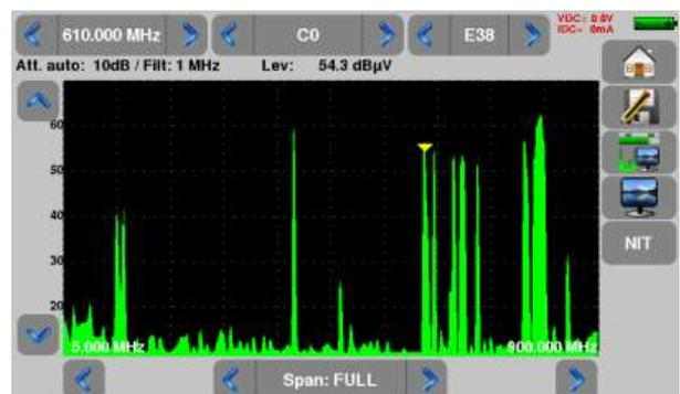
Press directly the signal you want in the spectrum (the cursor moves to where you press)
