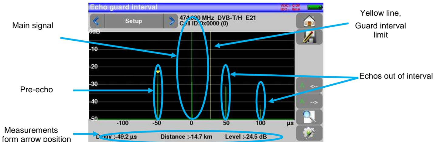
Relative amplitude in dB and delay in  $\mu\text{s}$  (distance in km) from the main signal (0 pulse) can be measured.
