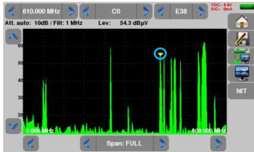
Press the NIT key
