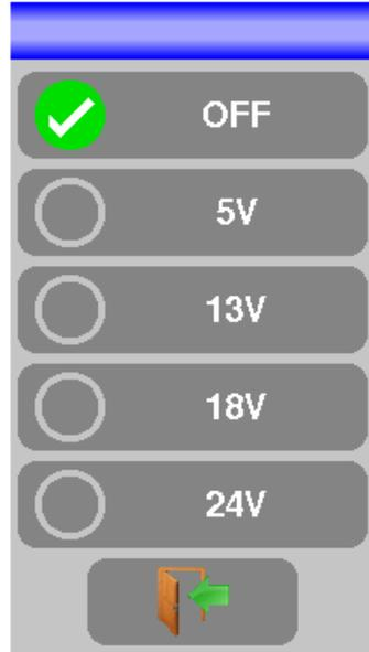
You can select the desired voltage by pushing on the correct button.
