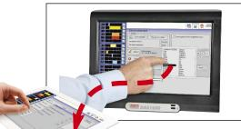
With Virtual Network Computing software, you remote control your DAS1600 from a computer or a tablet.
