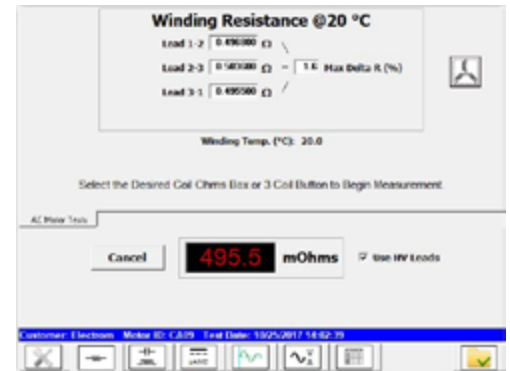
\mu\Omega measurement of 3-phase motor
