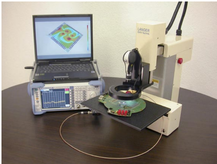
Test setup of IC Scanner FLS 102 with an universal PCB holder (UH-DUT).
