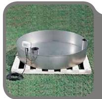
**Evaporimeter** LSI LASTEM evaporimeter pan and plastic platform are built to WMO
