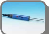
**Soil moisture sensor** DQA340 is the ideal solution for the measurement of volumetric moisture in soils and other porous materials. The sensor is based on TDR technology (Time Domain Reflectometry), ensuring good accuracy even in very wet soils, and without special calibration for mineral soils. Using its rods, the sensor can be inserted in the material for 11 cm. It measures both soil moisture (0-100% range) and temperature.
