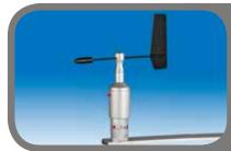
**Standard wind vane (analog output)** Wind direction sensor with analog signal output. All models use a Hall-effect encoding system. DNA811-815 are equipped with heaters to avoid ice formation on its body in very cold environments.
