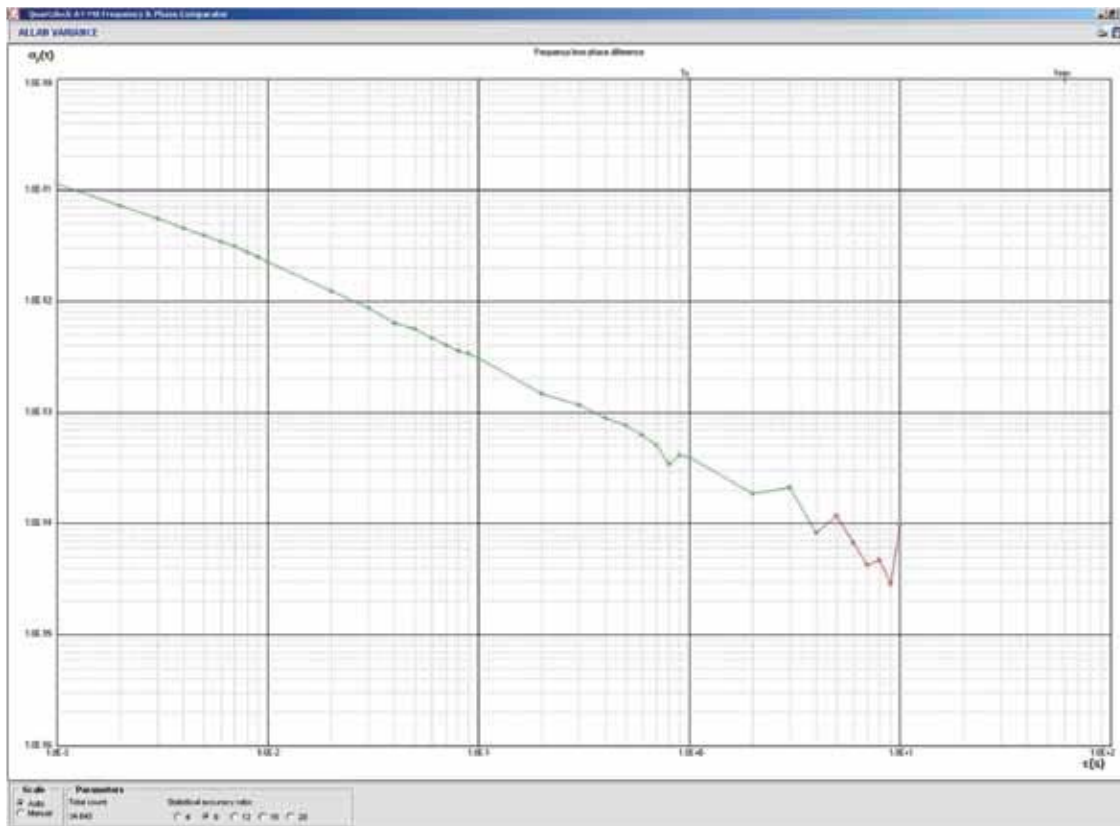
A7-MX Allan Variance (10MHz) – Narrowband high resolution mode. 10 -3 s to 10s (red plot is predicted)
