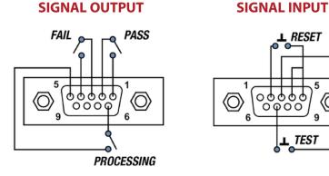
Figure 1 Pin Configurations for Remote I/O
