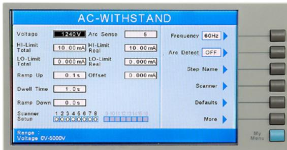
The above menu shows an OMNIA II connected to a 16-channel Scanner configuration. This configuration can be one external 16-channel Scanner (8 high voltage ports and 8 high current ports), or two external 8-channel Scanners. With two external 8-channel Scanners, one Scanner should be connected to the Scanner 1 connector on the rear panel of OMNIA II and the second Scanner should be connected to the Scanner 2 connector on the rear panel of OMNIA II.
