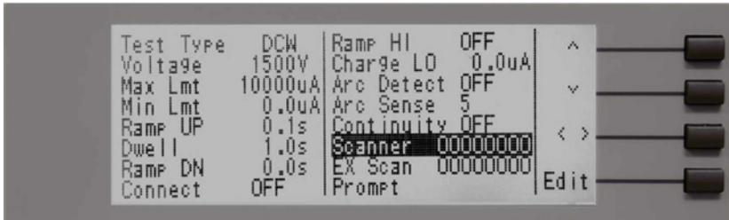
The above menu shows a HypotULTRA III with 16 Scanner channels (8 internal and 8 external). The "Scanner" parameter in the menu pertains to an internal 8-channel Scanner and the "Ex Scanner" parameter pertains to an 8-channel High Voltage SC6540 Scanner.
