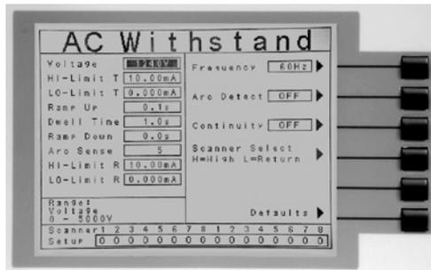
The above menu shows an OMNIA connected to a 16-channel Scanner configuration. This configuration can be one external 16-channel Scanner (8 high voltage ports and 8 high current ports), or two external 8-channel Scanners. With two external 8-channel Scanners, one Scanner should be connected to the Scanner 1 connector on the rear panel of the OMNIA and the second Scanner should be connected to the Scanner 2 connector on the rear panel of the OMNIA.
