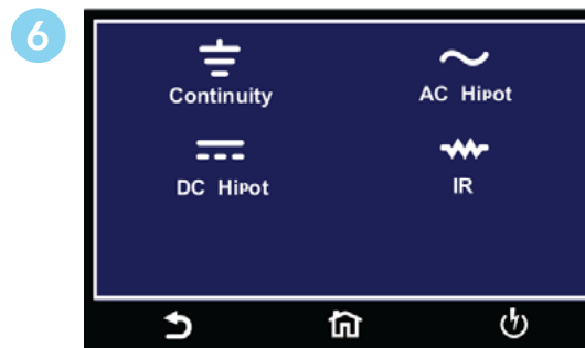
FailCHEK Menu - Check the instrument's failure detectors
